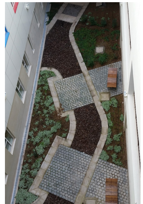
Floradrain® FD 25-E is used as permanent form-work for the separation between hard surface and garden.
